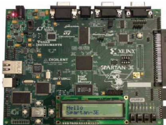
Figure 5.2: Spartan 3E FPGA Development Kit
