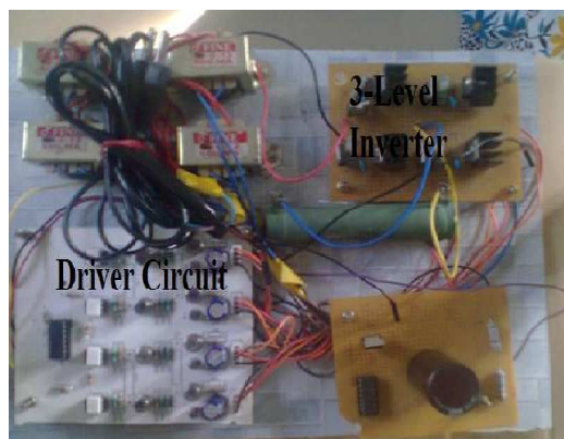
Figure 7.4: The Complete Hardware Circuit without Kit Connected
